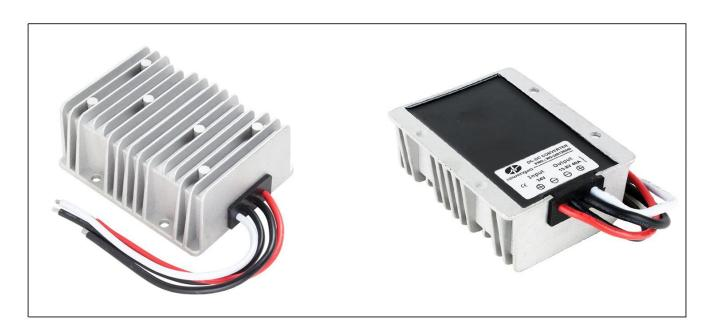
The WG-24S13R840 is a Non-isolated DC-DC converter that uses a synchronous rectification technology, and features high efficiency and power density. It has the dimensions of  $100 \text{mm} \times 80 \text{mm} \times 39 \text{mm}$  (3.94 in. x 3.15 in. x 1.54 in) and provides the rated output voltage of 13.8 V and the maximum output current of 40 A.
