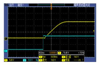
Figure 9, Short-circuit & Output voltage (Iout = 40A)
