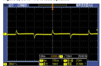
Figure 6, Output voltage established (Iout = 40A)
