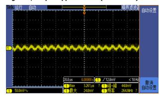
Figure 8, Boot delay time (Iout = 40A)
