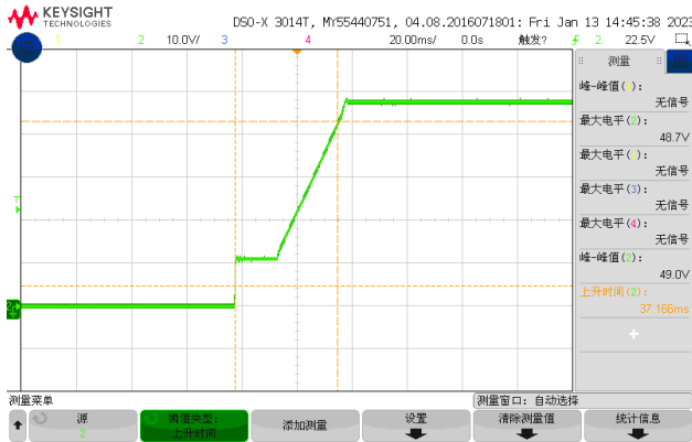
Figure 6, Output voltage established (Iout = 12.5A)
