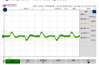
Figure 6, Output voltage established (Iout = 8A)
