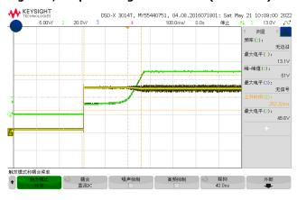
Figure 7, Output ripple & noise (Iout = 8A)
