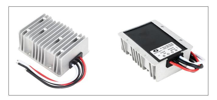
The WG-12S4808 is a Non-isolated DC-DC converter that uses a synchronous rectification technology, and features high efficiency and power density. It has the dimensions of  $100 \text{mm} \times 80 \text{mm} \times 39 \text{mm}$  (3.94 in. x 3.15 in. x 1.54 in) and provides the rated output voltage of 48V and the maximum output current of 8A.
