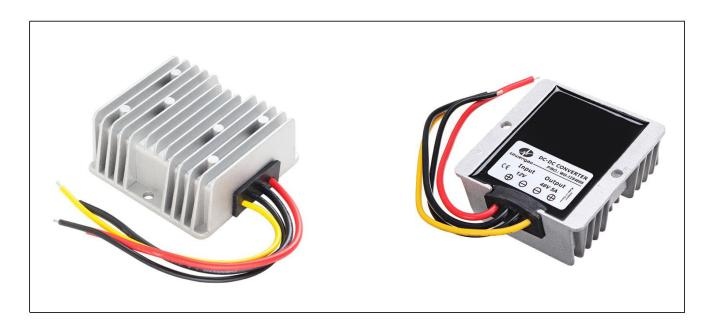
The WG-12S4805 is a Non-isolated DC-DC converter that uses a synchronous rectification technology, and features high efficiency and power density. It has the dimensions of  $74 \, \text{mm} \times 74 \, \text{mm} \times 32 \, \text{mm}$  (2.91 in.  $\times 2.91$  in.  $\times 1.26$  in) and provides the rated output voltage of  $48 \, \text{V}$  and the maximum output current of 5A.
