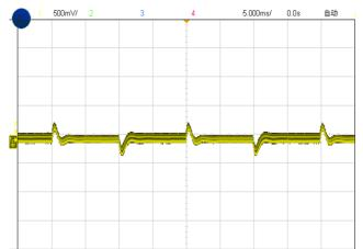
Figure 6, Output voltage established (Iout = 5A)
