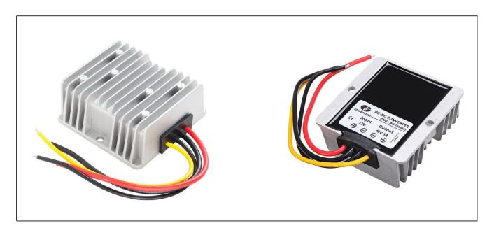
The WG-12S4803 is a Non-isolated DC-DC converter that uses a synchronous rectification technology, and features high efficiency and power density. It has the dimensions of  $74 \, \text{mm} \times 74 \, \text{mm} \times 32 \, \text{mm}$  (2.91 in.  $\times 2.91$  in.  $\times 1.26$  in) and provides the rated output voltage of  $48 \, \text{V}$  and the maximum output current of  $3 \, \text{A}$ .
