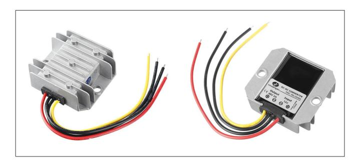
The WG-12S4802 is a Non-isolated DC/DC boost converter that uses a synchronous rectification technology, and features high efficiency and power density. It has the dimensions of 64mm x 57mm x 22mm (2.52 in. x 2.24 in. x 0.86 in) and provides the rated output voltage of 48 V and the maximum output current of 2A.
