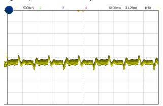
Figure 6, Output voltage established (Iout = 2A)
