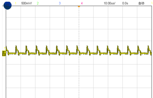
Figure 7, Output ripple & noise (Iout = 1A)
